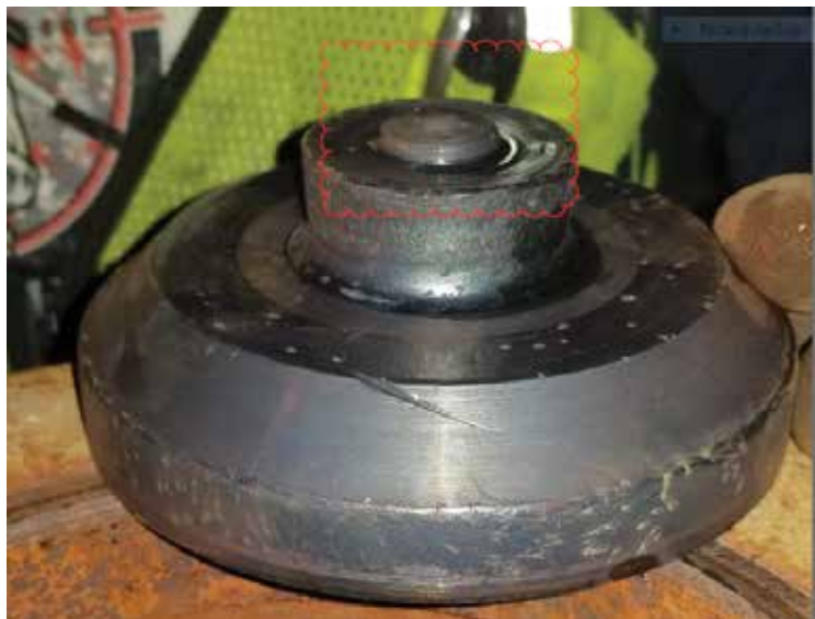
Figure 1: Swing check valve disc stud failure caused by chattering
