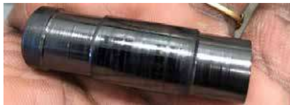
Figure 3: Undue wear of hinge pin in a swing check valve due to chattering
