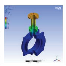
temperature, the valve is disassembled and the pressure retaining parts are examined for defects. These are similar to the conditions the valve will be subjected to during its normal operation.
