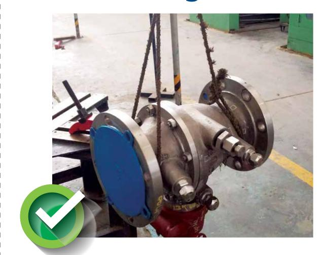
Lift using ropes/belts around the body
