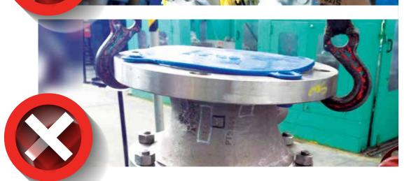
Do not lift using yoke or hand-wheel Do not use hooks on the flange
