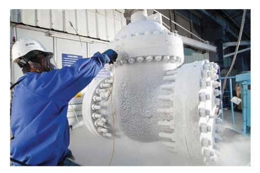
With 6 active cryogenic valve standards in the industry, it is important to understand the requirements spelt out in each of these standards. The standards differ in terms of the extension lengths for cold box and non-cold box applications, drip plate design, stem strength guidelines, test sequence, number of cycles, to name a few. Figure 1 shows the scope and applicability of the various cryogenic valve standards.
