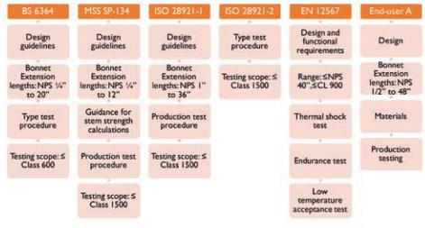
Figure 1 - scope and applicability of the various cryogenic valve standards/specifications
