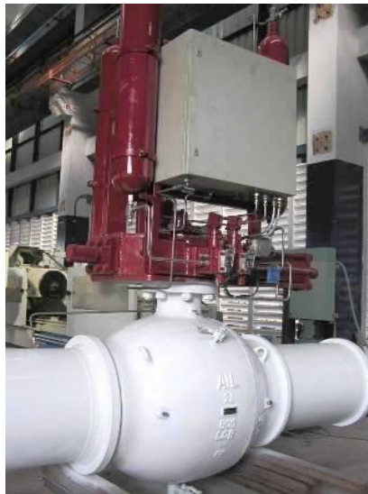
Fig. 5 - L&T TMBV with Gas over oil actuator
