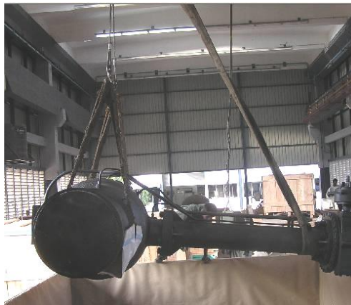
Fig. 9 - Handling a welded end valve with an extended stem
