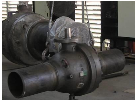
Fig. 3 - Handling a valve with welded pup piece.
