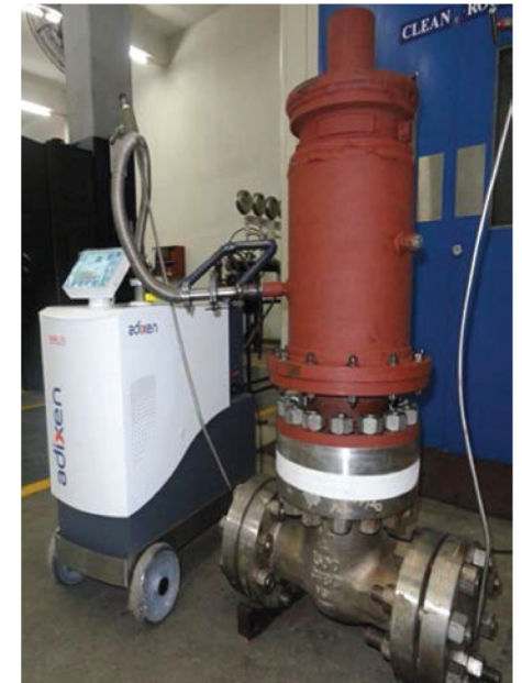
Figure 2: ISO 15848-1 Vacuum method - Global measurement
