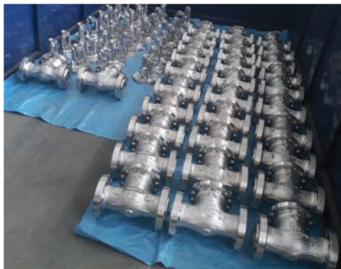
Castings lined up for TPI.
