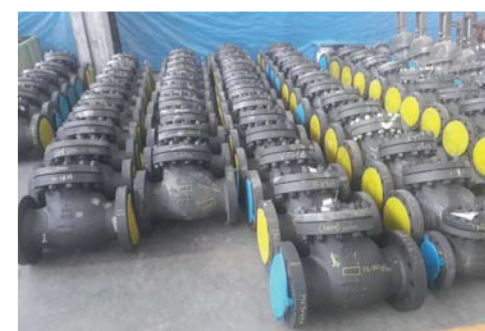
Valves internally tested OK lined up for hydrotest offering to TPI.
